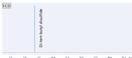
Simultaneous Analysis of Sulfur Standard Components in Diesel Using GC-MS and SCD
