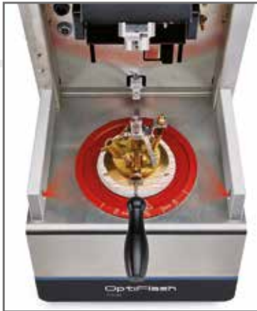
Optical fire detecting system covers entire hot area
