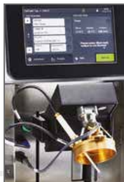
Lift-arm and touch-screen make it easy to operate
