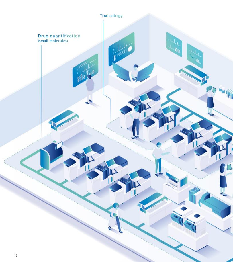
From the sample tube, the CLAM can perform extraction and LC/MS analysis automatically.
