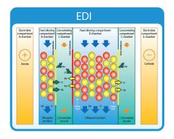
components within a water system. The resin within the cell is continuously regenerated by virtue of the electrical current.
