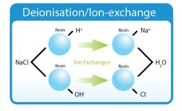
quaternary amino groups such as polyAPTAC to exchange a hydroxyl for any anions (e.g. Cl-,  $NO_3$ - ,  $SO_4$ -). When the hydrogen ion from the cation exchanger unites with the hydroxyl ion of the anion exchanger pure water is formed.
