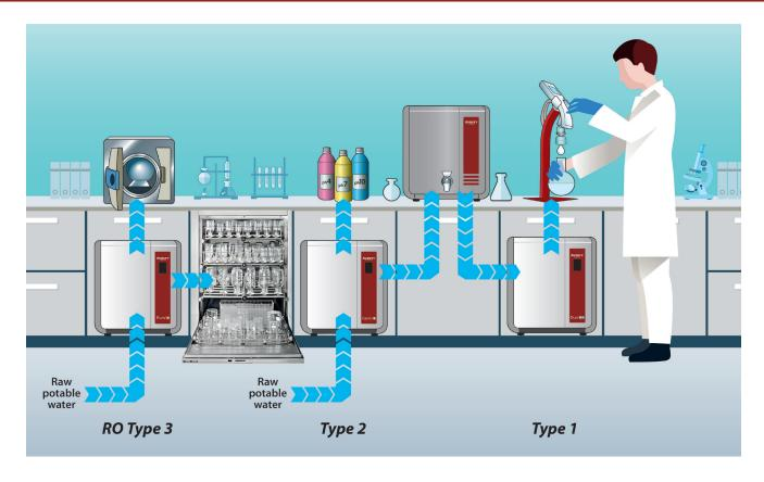
Pure water systems can be constructed using modular, off-the-shelf components to minimise cost and maximise compliance and validation efficiency. Component selection should be carefully considered.
