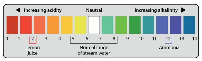
It is commonly believed that the pH of ultrapure water should be a neutral 7.0. In fact, ultrapure water pH can decrease rapidly immediately after being dispensed from a laboratory water system due to absorption of CO<sub>2</sub> which creates carbonic acid and causes the pH level to drop to an acidic pH.
