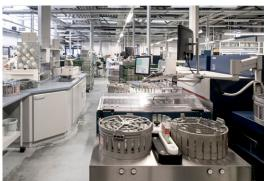
Based on Individual Bacteria Count (IBC), BactoScan™ FC+ gives an accurate determination of the hygienic quality of raw milk with a capacity of testing up to 200 samples per hour. BactoScan is the industrial standard in many countries all over the world, and in the EU more than 75% of all milk supplies are paid based on BactoScan results.
