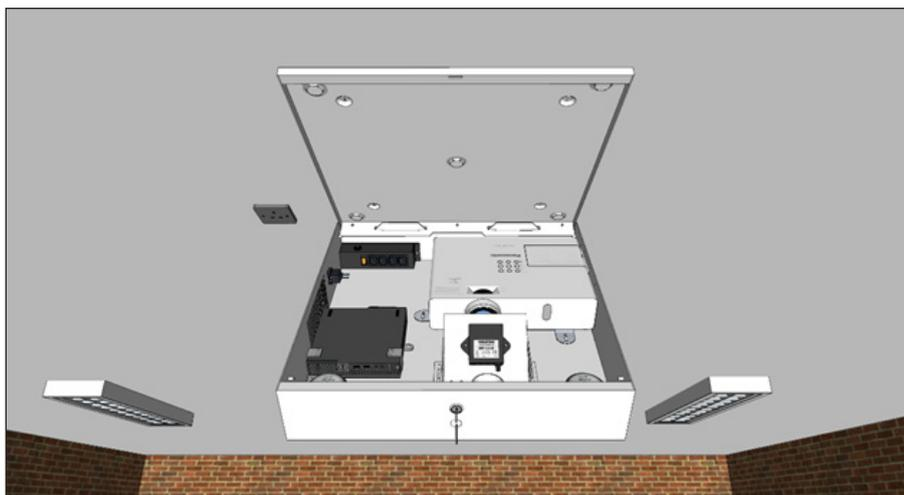
Once the main unit is closed to the ceiling plate, the security strip must be fitted to the back of the ceiling plate using 3 x M4 Screws (supplied) to prevent accidental separation of the main unit from the ceiling plate.
