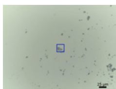
Observation image of the foreign matter on the diamond cell by 15x Cassegrain objective mirror.
