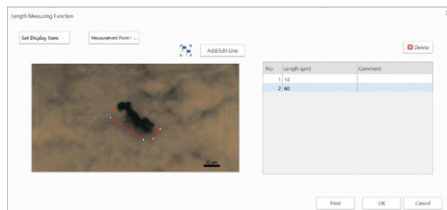
Measurement screen using length measurement function
