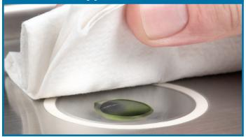
Some manufacturers use glass or YAG ( Yttrium-Aluminum-Garnet.) prisms. These prisms are softer than synthetic sapphire and have slower temperature transfer coefficients.
