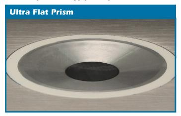
**Easy to clean prism** – No matter how good the refractometer is, the results will only be right if the prism is clean. **Rudolph's flat prism sample well interface design makes cleaning easy**, even with sticky syrups. The flat low profile sample well with a sample volume of less than 1ml is easily cleaned by wiping with a common paper towel. A single cleaning surface with a **scratch-proof synthetic sapphire prism** makes the J157 a popular choice for high throughput laboratories.
