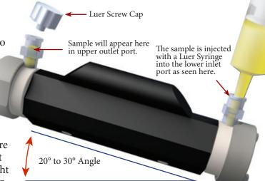
Syringe. When the sample appears near the top outlet port, simply place the Luer cap on the upper port and then lower port. Your cell is now filled, capped and air bubble free. Cells must be clean and dry to ensure proper filling with minimum sample.
