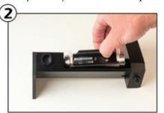
Place a 2.5mm or 5.0mm bore Polarimeter cell into the Rudolph FillStation<sup>TM</sup>.
