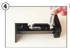
Make sure the cell is always clean and dry. Use compressed air and acetone for this process. Fill the cell from the lower inlet port with a Luer Syringe only. As the cell becomes filled and sample begins to appear at the upper inlet, cap off the upper then lower inlet port. Your cell is now filled and air bubble free.
