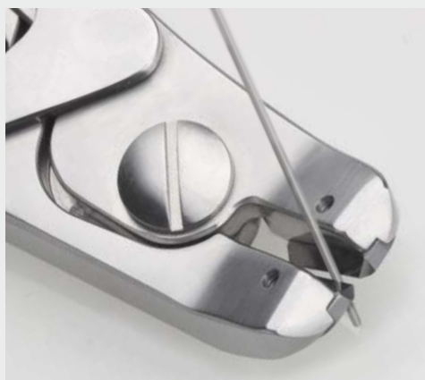
Cutting K-wire with the EasyCut
