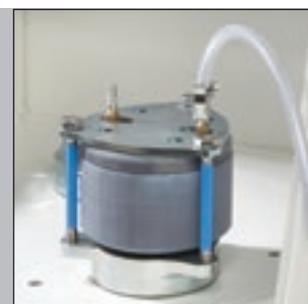
The PULVERISETTE 4 grinding in inert gas
