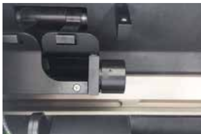
Built-In quartz plates will perform a 3 point validation automatically.
